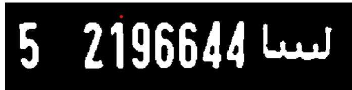
Fig. 20. License plate image after removing small objects.
